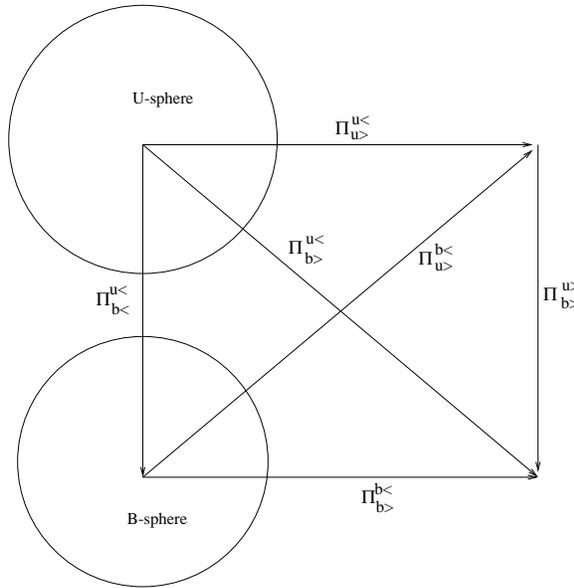
**Figure 1.** Various energy cascade rates of MHD turbulence. The illustrated wave-number spheres contain  $\mathbf{u} <$  and  $\mathbf{b} <$  modes, while  $\mathbf{u} >$  and  $\mathbf{b} >$  are modes outside these spheres. The velocity field is forced at large-scale.
