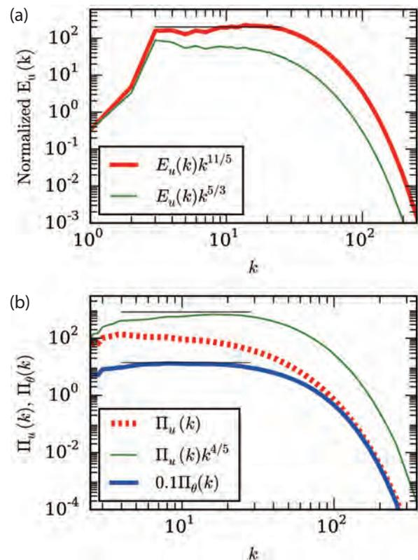
**Fig. 2:** For stably stratified turbulence plots of (a) normalized kinetic energy spectra  $E_u(k)$  with  $k^{-11/5}$  and  $k^{-5/3}$  and (b) kinetic energy flux  $\Pi_u(k)$ , normalized KE flux  $\Pi_u(k)k^{4/5}$ , and potential energy flux  $\Pi_\theta(k)$ .
