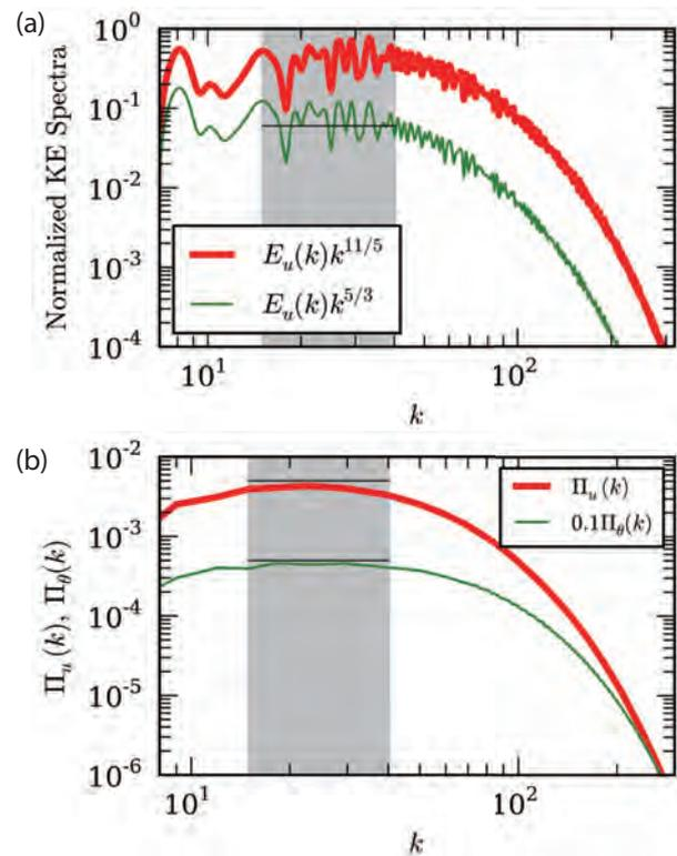
**Fig. 3:** For RBC simulation (a) plots of normalized KE spectra for Bolgiano-Obukhov scaling and Kolmogorov scaling; (b) KE flux  $\Pi_u(k)$  and entropy flux  $\Pi_\theta(k)$ . The shaded region shows the inertial range.
